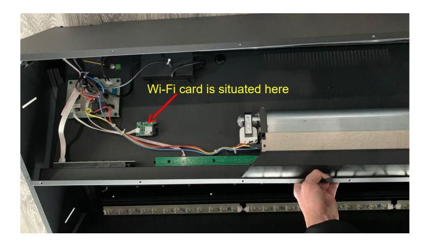
**Step 3** To replace a new WiFi card, remove the screws circled in red and unplug the old one .
