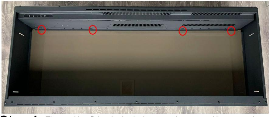
**Step 1** The steel bar fixing the back glass must be removed by unscrewing the screws circled in red. The back glass can then be removed
