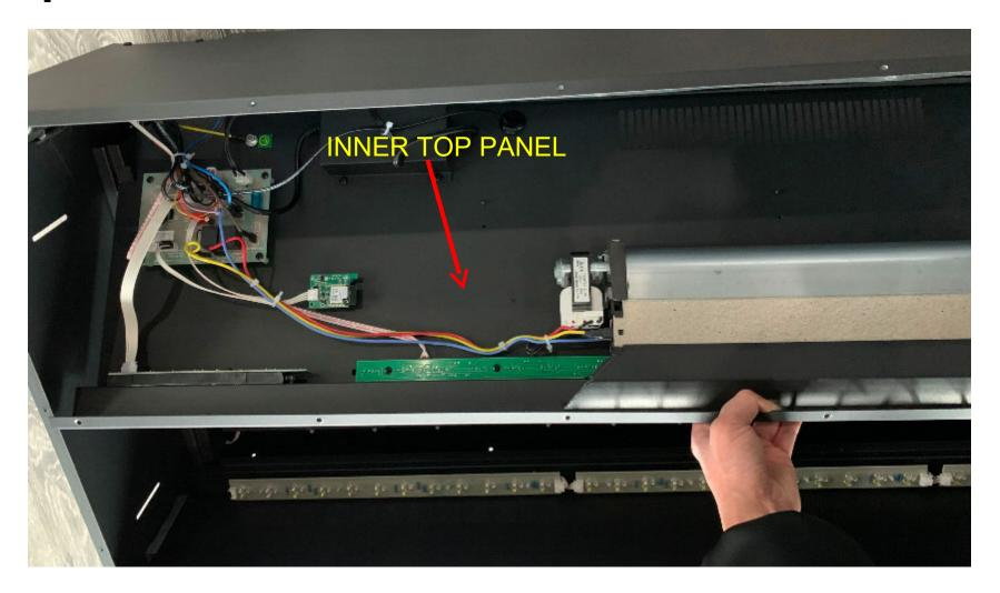
**Step 5** Unplug the flicker motor from the circuit board and replace it with a new one.
