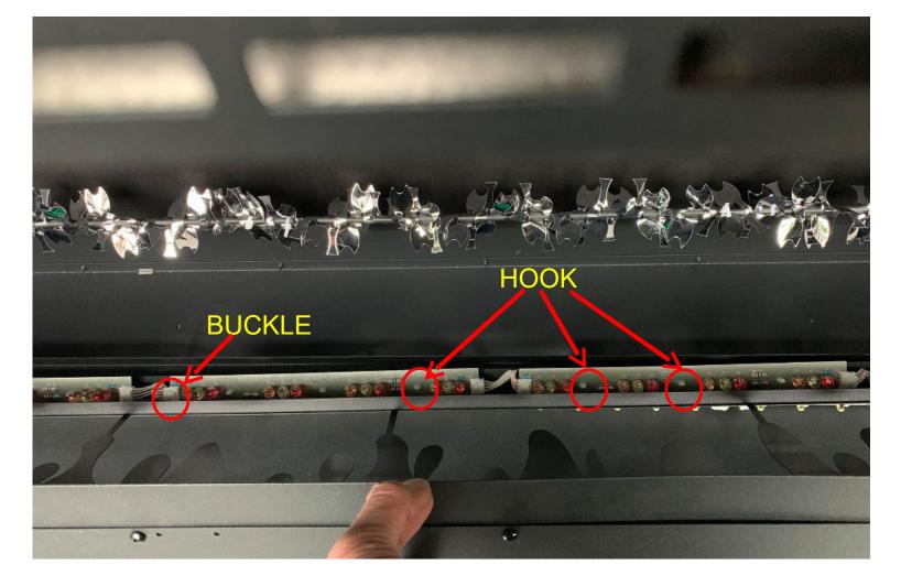
**Step 3** The defective LED strip must be removed from the hooks and the buckle must be unplugged to replace it
