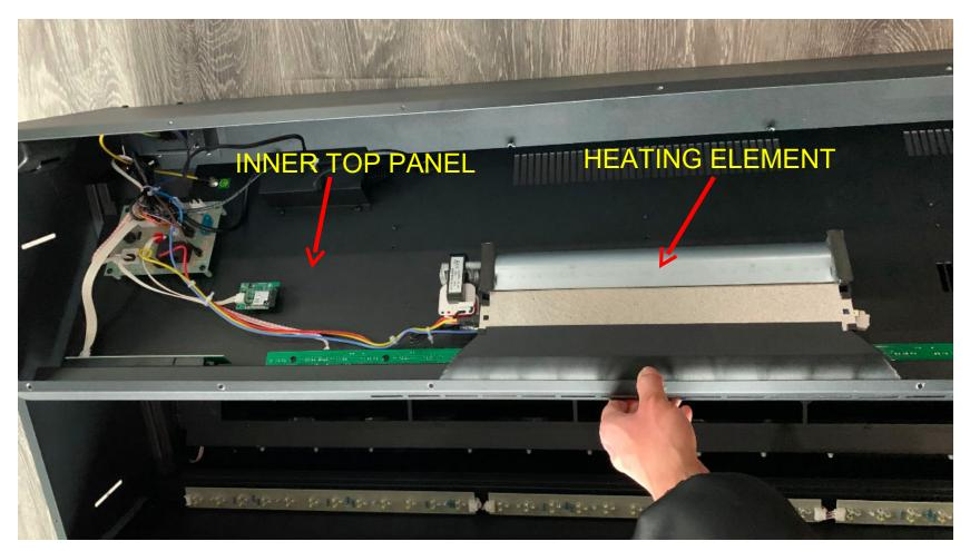
PLEASE NOTE for SYM-60/74/88/100-XT(120V model), there are 2 sets heating elements, the repair procedure remains the same.
